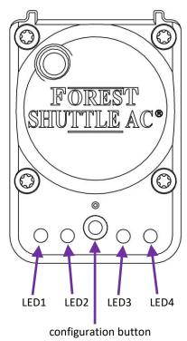
Use a pin to change settings in the configuration menu. Choose the setting you want to change (table below) and press the button that many times (corresponding with setting).
